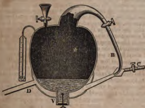
No. 221. Apparatus for evaporating liquids in vacuo.
